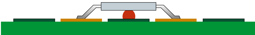
Figure 8.11 Aperture modifications to increase GDH
