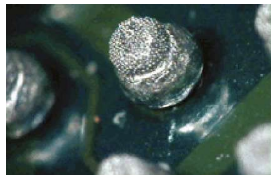
Figure 7.16 Results from a 0.150mm direct printing rework stencil
