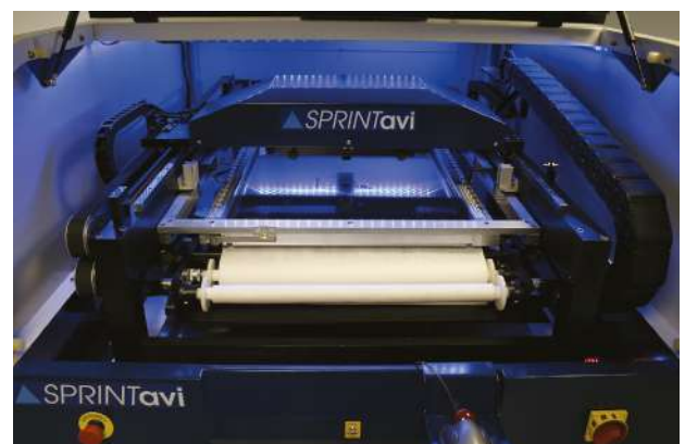
Figure 4.28 Under-stencil cleaning mechanism
