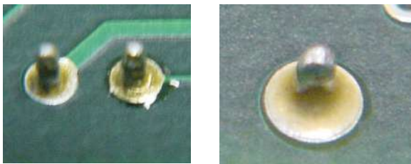
Figure 8.43 PIHR solder fillets seen from the underside of the PCB
