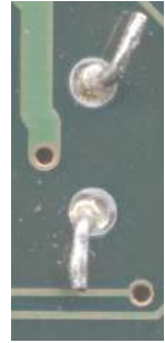
Figure 8.40 2-pin inductor with uncropped legs
