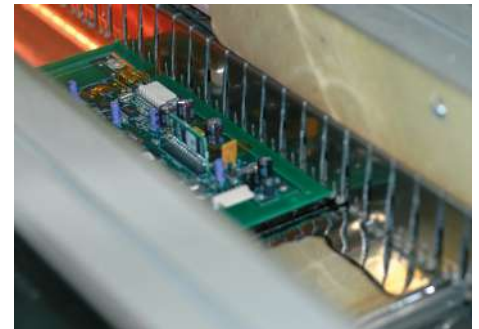
Figure 8.4 PCB entering solder wave
