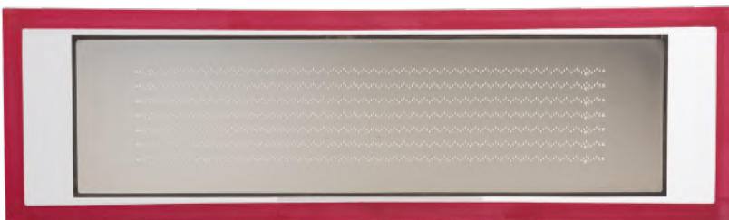
Figure 2.5 Extended stencil meshed into aluminum frame
