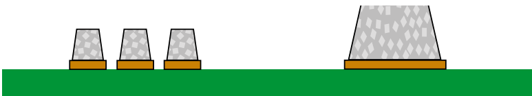
Figure 6.39 Selective multi-height paste deposits can be achieved using multi-level stencils
