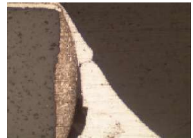
Figure 6.20 Cracked solder fillet
